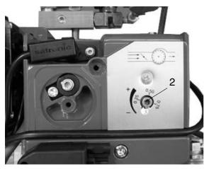
Setting the combustion air flow rate (2).
