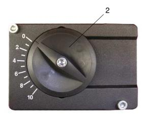
Setting the combustion air flow rate (2).
