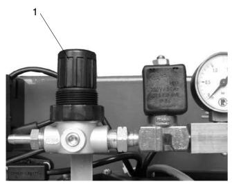
The primary airflow should be set using the pressure regulator (1) according to the required burner output. The information given in the diagram can be used as guide values.
