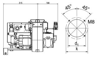
X= Burner tube extension 100 mm and 200 mm
