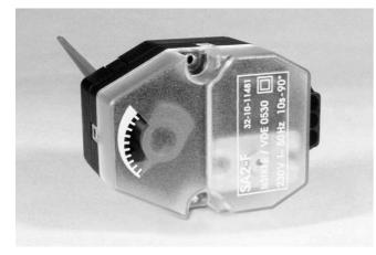
On version -L burners an air damper prevents the furnace from cooling down when there is a burner stoppage. Control of the air damper is effected electrically. The air flap opens before the burner starts. Its position can be read off the servomotor.
