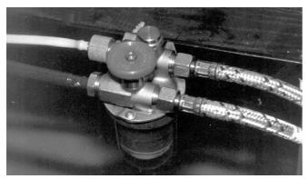
For pure single-pipe operation the bypass stopper must be unscrewed out of the return line opening and the return line opening must be sealed with a gasket and metal stopper.
