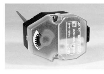
On version -L burners an air damper prevents the furnace from cooling down when there is a burner stoppage. Control of the air damper is effected electrically. The air flap opens before the burner starts. Its position can be read off the servomotor.
