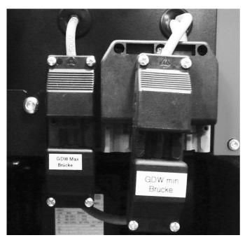
The gas pressure switch MIN at the gas fitting serves to monitor the gas inlet pressure. If the minimum gas inlet pressure is not reached (factory setting), the burner is switched off. The burner automatically starts again when the minimum pressure is exceeded. The gas pressure monitor as density control DK generally serves to check the valves and must be set to 50% of the static gas inlet pressure.
