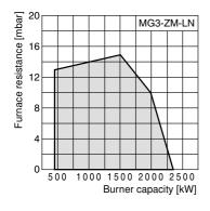
Working range acc. to DIN EN 676. The working range is referred to 15°C and 1013 mbar.
