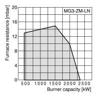
Working range acc. to DIN EN 676. The working range is referred to 15°C and 1013 mbar.
