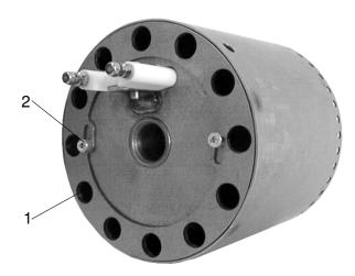
The design and mode of operation of the mixing unit used takes account of the basic connections between flow, combustion and the generation of pollutants. In addition to the setting of the dimension "A" de-
