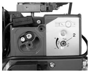
Setting the combustion air flow rate (2).
