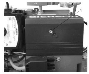
Undo screw (1) using Allen key (size 4) and remove cover.
