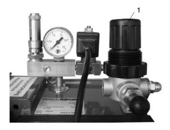
The primary airflow should be set using the pressure regulator (1) according to the required burner output. The information given in the diagram can be used as guide values.
