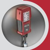
Hands free operation with magnet power using the 4 magnets from analyser rear side, this one will firmly stick on ferous surface.
